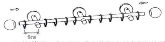
5. Once the pole is position on the brackets and in the correct place, tighten down the screw on the top of the bracket with a hex key provided until it is holding the pole in place.
